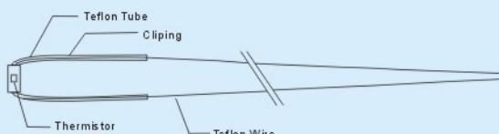
**Operating Temp. Range****-20 to +180°C****Dissipation Constant****Approx. 3 mW/°C (still air)****Response Time****Approx. 12 sec. (thermal bath)**
