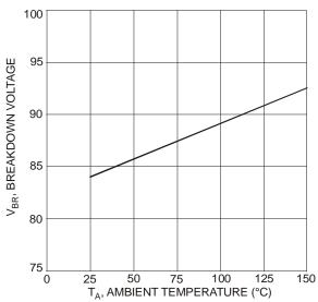
Fig. 4 Average Breakdown Voltage vs. Ambient Temperature
