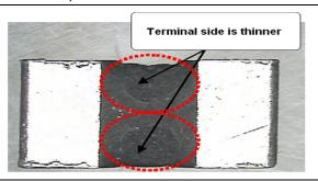
10.3.2 When customer performs wave solder process shall take note on the dispensing gap. If the gap between two dispensing is over, the red-glue will not adhesive the resistor body and be dropped out (as photo 1). Therefore, we suggest customer to narrow down the dispenser gap (as photo 2), or dispenser on the body center (as photo 3)
