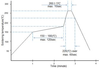
Recommended IR Reflow Soldering Profile MEET J-STD-020D
