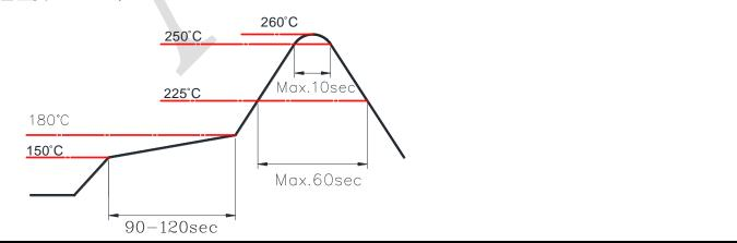
**Soldering with iron** Hand Soldering :  $360\pm10^{\circ}$ C /  $\leq$  2 Sec.
