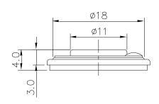
The speaker which meet waterproof standard IP 65 for Protection from a jet of water from all direction.
