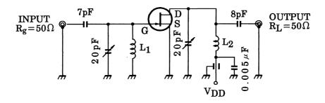
L1: 0.8 mm $\phi$  Ag plated Cu wire 3 turns, 10 mm ID, 10 mm length
